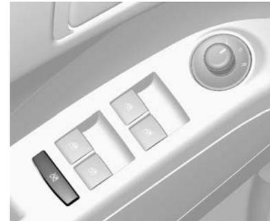
Pressione o interruptor
